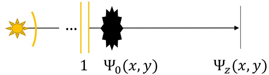
The use of serrated external occulter in stellar and solar coronagraphy comes from very different reasoning, but the diffraction principle is the same
