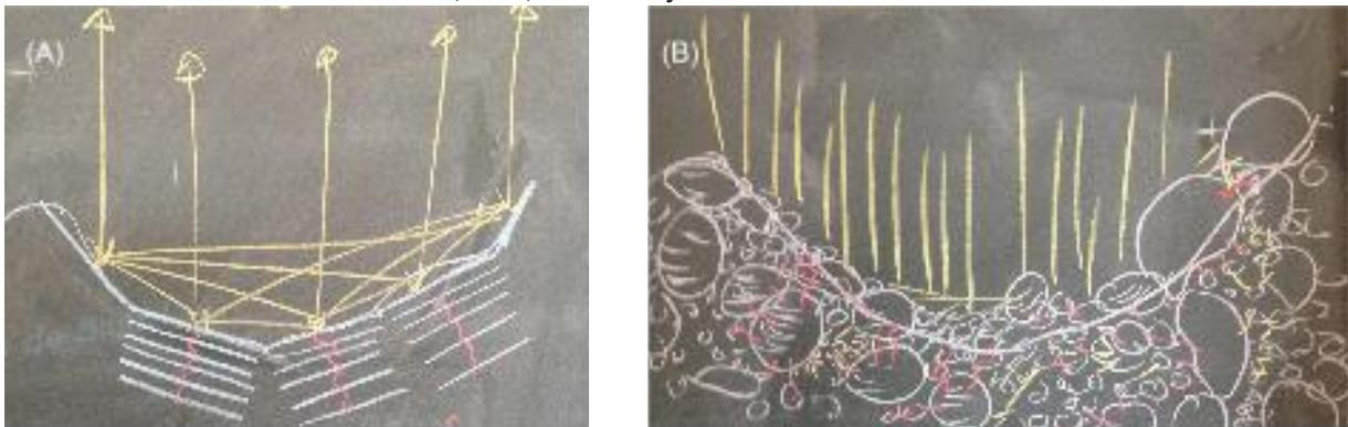
Figure 3: We want to pass from (A) the simple TPMs that treat 1D **heat conduction** in the subsurface of planar facets and **radiative transfer** to space and mutual facets heating, to (B) a physically based model of heat transfer into a multi-dispersed granular medium (regolith) with local 3D **heat conduction** and **radiative transfer**. Note that in the TPM there is no lateral **conduction**. Sketched here is e.g. a crater wall.
