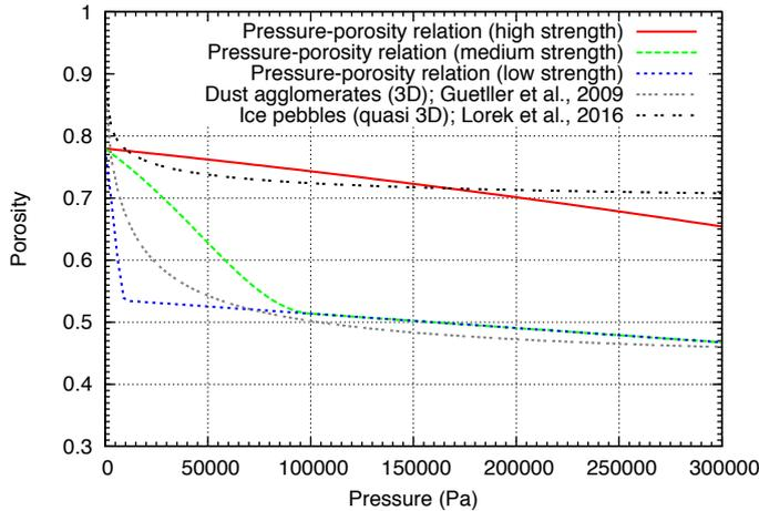
**Fig. 1.** Pressure-porosity relations (crush curve) used in the simulations for the three different sets of parameters (low, medium, high strength) as defined in Table 1. Also shown are the results from laboratory experiments dust agglomerates (Güttler et al. 2009) and ice pebbles (Lorek et al. 2016).
