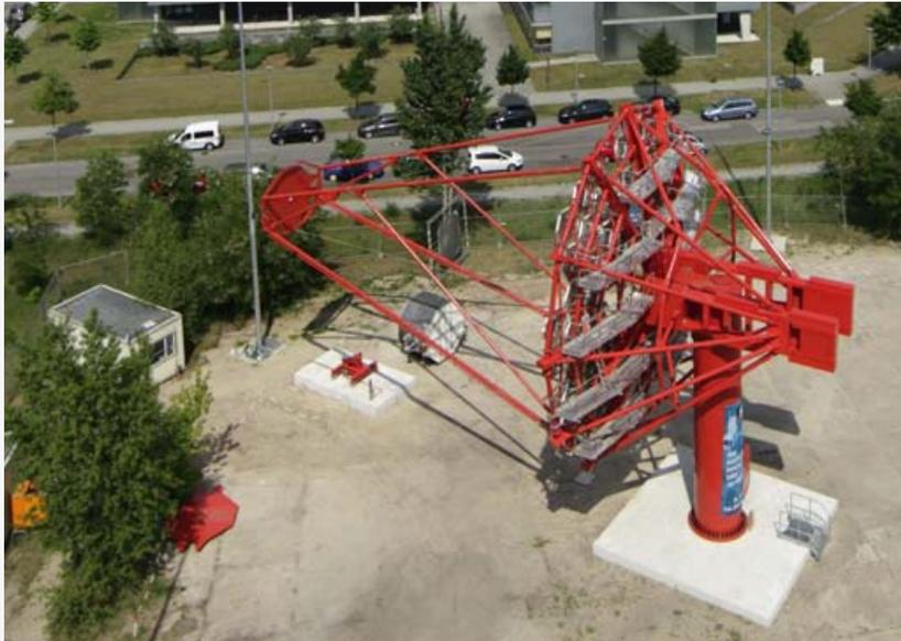
**A prototype for the 12-meter medium-size CTA telescopes, built at DESY in Berlin/Zeuthen**
