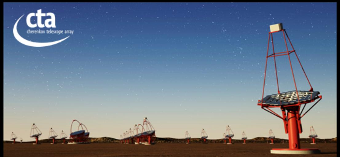
With telescopes distributed over a few  $\text{km}^2$ , the *Cherenkov Telescope Array* can operate as a kilometric optical intensity interferometer to achieve diffraction-limited imaging and optical aperture synthesis
