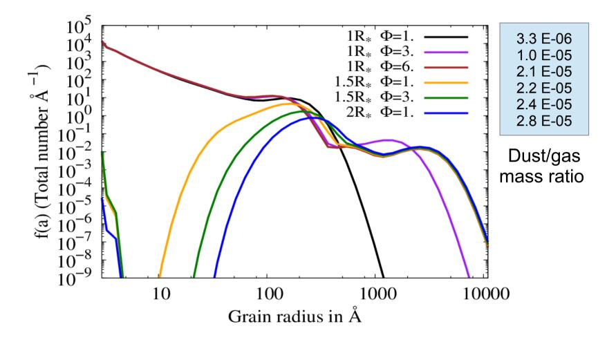
Large grains > 0.02 µm are already formed at 1, because gas densities are high in the postshock gas
