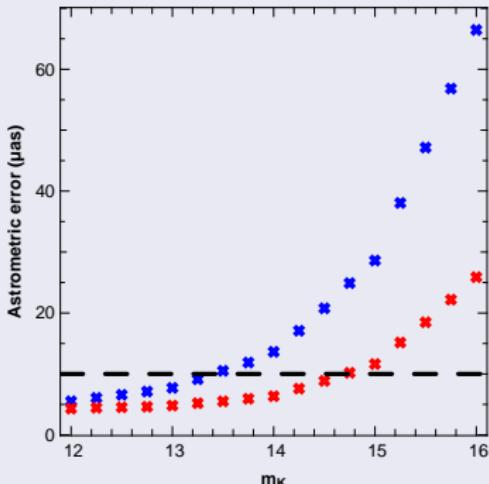
Errors in the direction of the **major** and **minor** axes of the PSF
