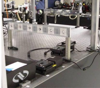
7. On a CHARA laptop, select the “BEAM SAMPLER” GUI (see Sect. 7). Use the information of the right column to configure each of the beams on their current position (memory of the position in fact). Then in the “ALL” box, select B5 and click on SET. All the beam samplers are sent to the B5 position so that the laser could be seen on the East table CHARA target.
