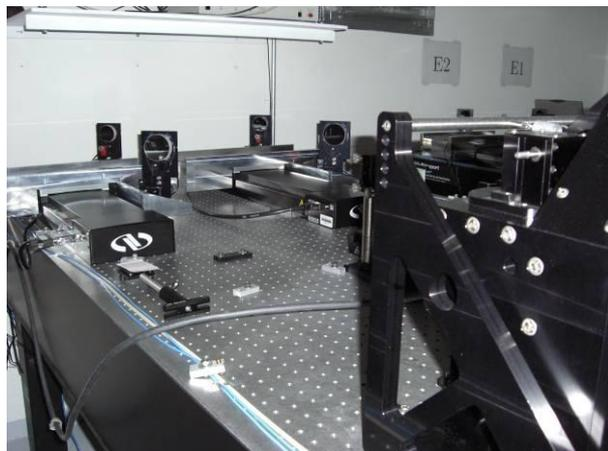
**Figure 4: interface for beam splitters and picture of the beam splitter**
