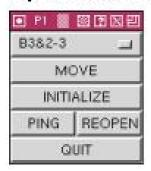
The first button allows you to select B6. When B6 is selected hit MOVE, this pops up a new window, which allows you to move the beam.
