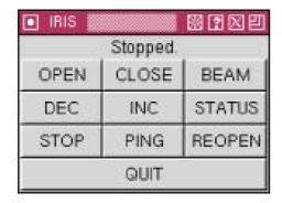
DEC = Decrease by one step INC = Increase by one step BEAM => Homes (closes) and sets it to the nominal beam diameter = 19 mm
