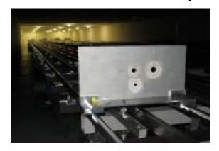
Place the rail target on the rail near the home sensor at the front.
