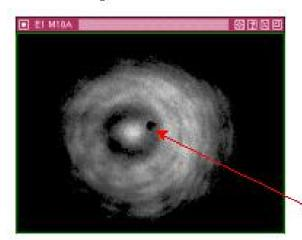
If the center of the diffraction pattern is not as well defined as in this picture, adjust the iris.
